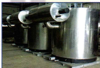
Flake Ice Generator
